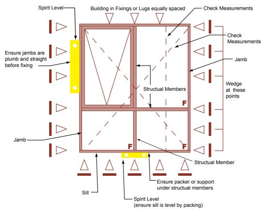
\* Fix via building lugs, nails or shim at equally spaced arrow points.
